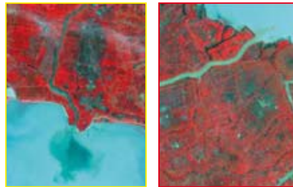
In Hefei basin, the colder waters from the southern river inlet are evident, while two rivers entering the lake's northern and western parts do not produce any anomaly. On the left, the thermal image (temperature increase from blue to red) is derived from ASTER TIR data acquired in June 2003. The false-color images show the land use close to the rivers entering into the Hefei basin.
