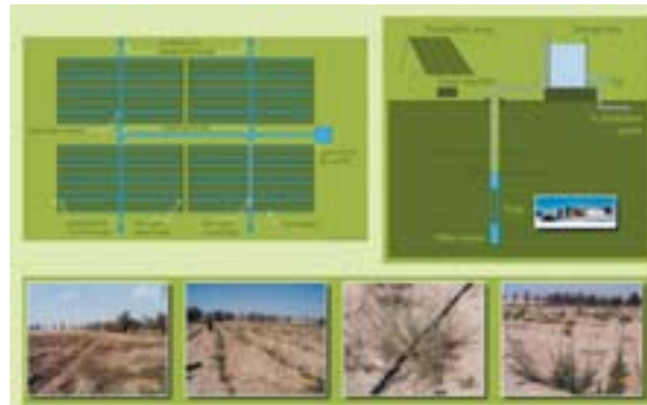
Layout of the drip irrigation system and a sketch of the solar pumping system (top). Details of the installation (bottom).
